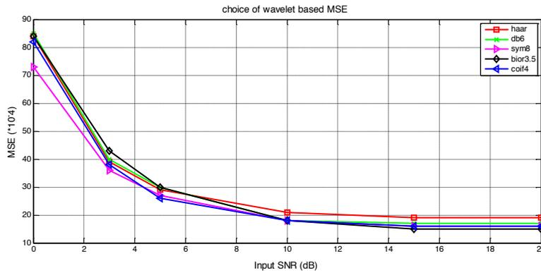
Fig. 10. Comparison MSE for different wavelet function
