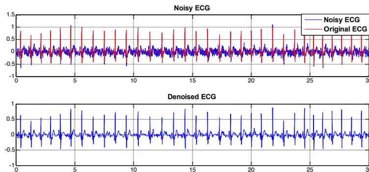
Fig. 15. Removal of EMG noise simulation
