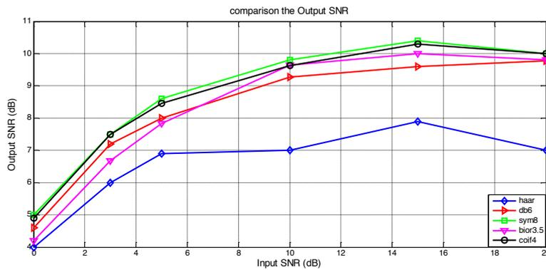
Fig. 8. Comparison output SNR for different wavelet functions with soft threshold
