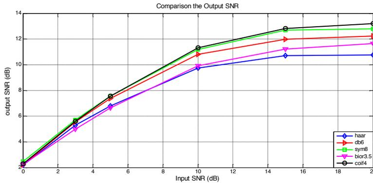
Fig. 9. Comparison output SNR for different wavelet functions with hard threshold
