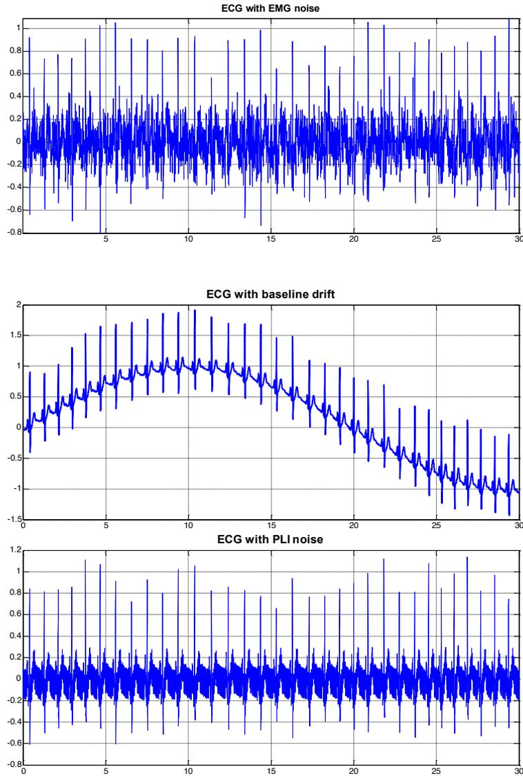
**Fig. 3.** Different types of noisy ECG signal
