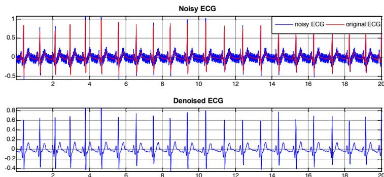
Fig. 17. Removal of PLI noise
