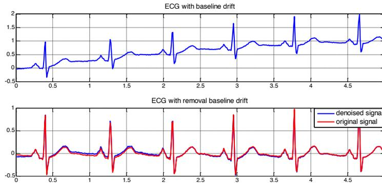
**Fig. 16.**Simulation of baseline drift correction
