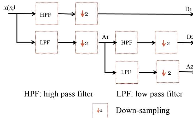
Fig. 4. DWT decomposition filter model
