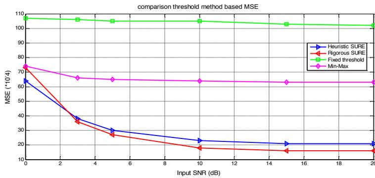
Fig. 12. Comparison MSE for different threshold methods
