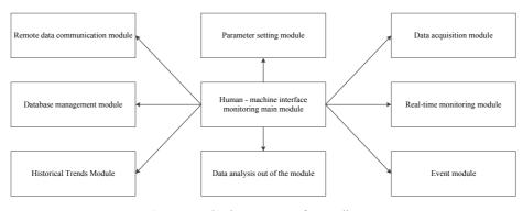
Fig. 5. Monitoring system software diagram
