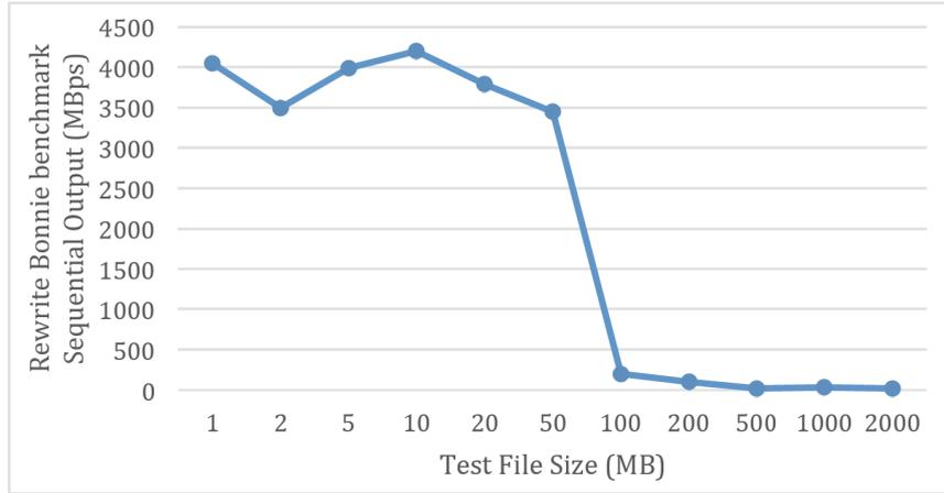
**Fig. 3.** Bonnie rewrite benchmark result. The performance drop indicate the capacity of memory-based disk cache
