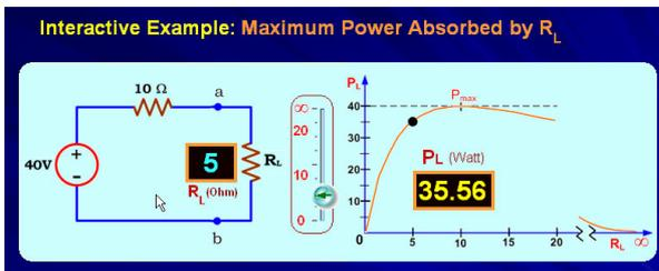
Figure 2. Interactive example on Maximum Power Transfer
