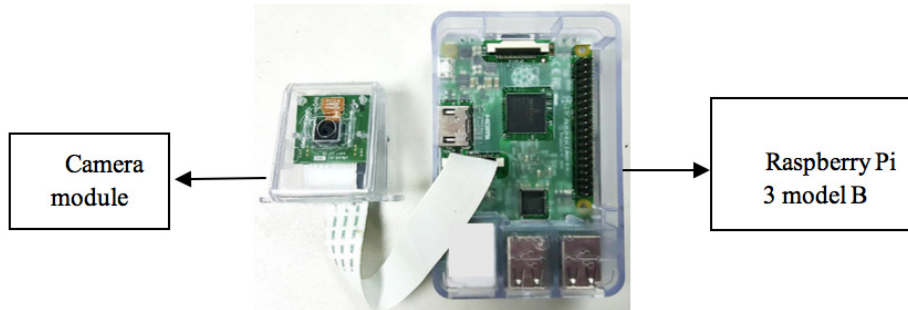
Fig. 2. Raspberry PI 3 model B board and camera module
