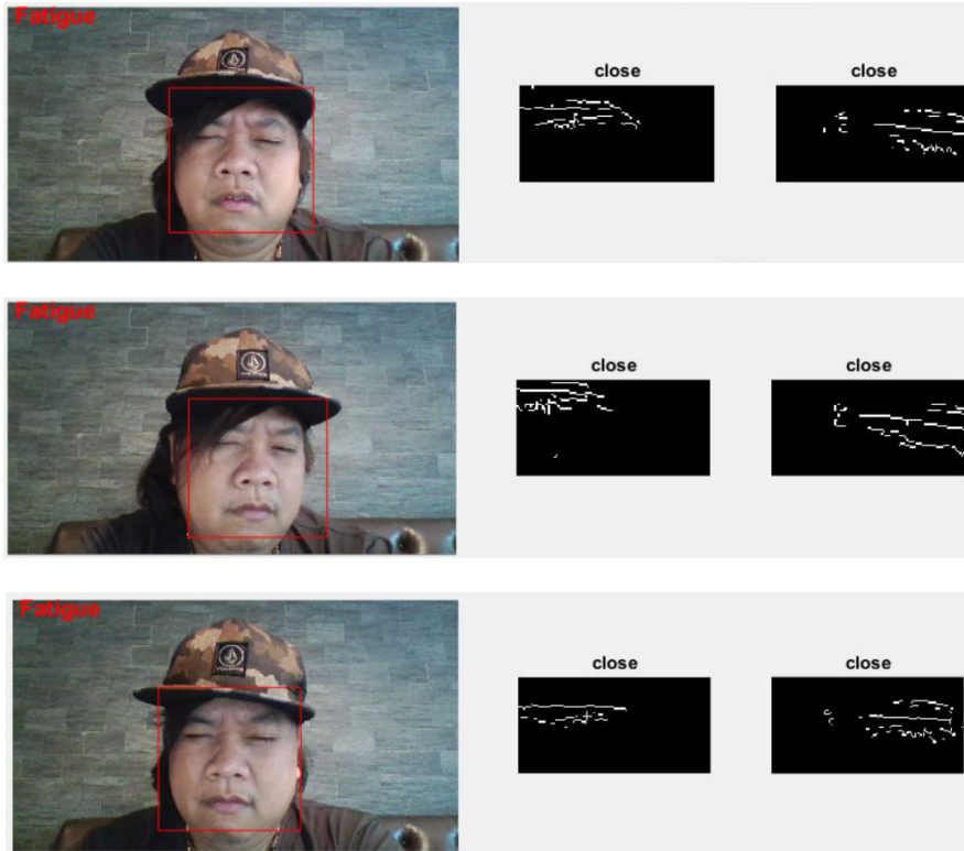
Fig. 15. Experimental Results of Eye-Closing Classification.
