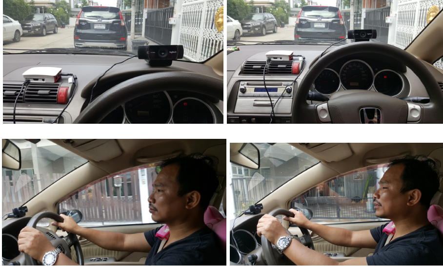
Fig. 18. Fatigue Monitoring System Installation
