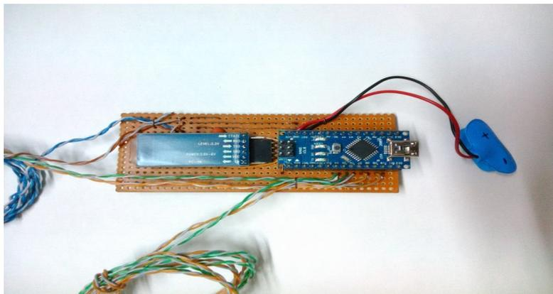
Fig. 5. Bluetooth module connection of the stick
