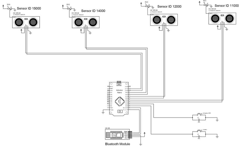
Fig. 2. Simulation of the blind stick via Proteus 8.0
