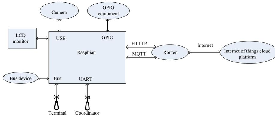
Fig. 2. The overall structure of the gateway
