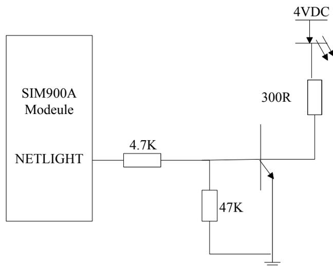
Fig. 4. Network status indication circuit
