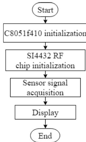
**Fig. 2.** The main flow of the sensor node
