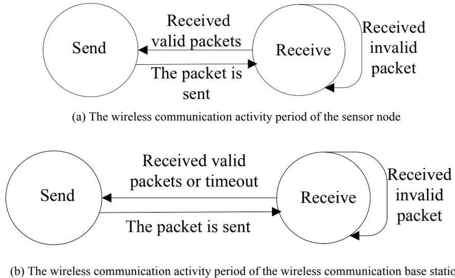
**Fig. 1.** The activity period of the sensor node and the wireless communication base station
