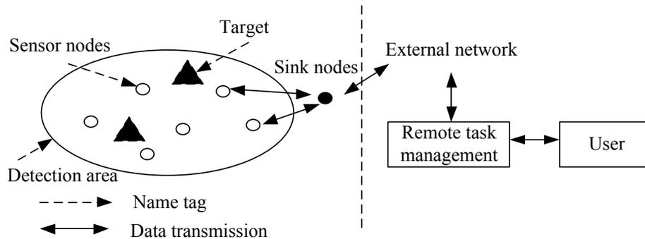
Fig. 1. Structure of wireless sensor network system
