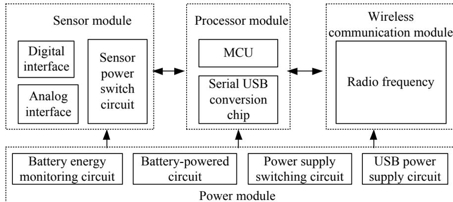
Fig. 3. The overall framework of hardware framework of sensor node
