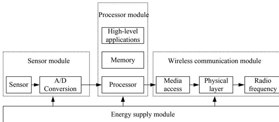
**Fig. 2.** Structure of wireless sensor network node system
