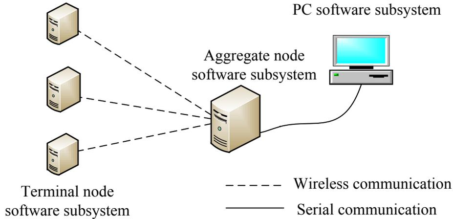
Fig. 4. The software system of wireless sensor network node
