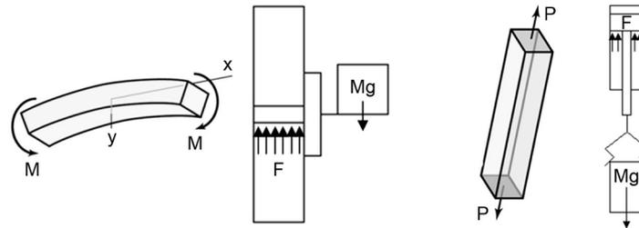
**Fig. 3.** Type of load – bending (left) and straining (right)
