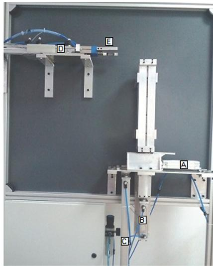
Fig. 1. The basic version of pneumatic circular manipulator
