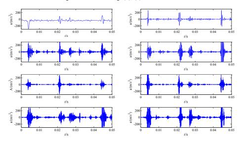
Fig. 7. Wavelet packet reconstitution signals of loose slipper fault
