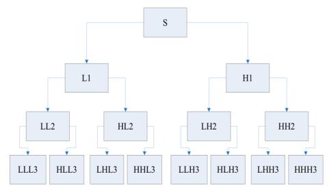
Fig. 1. 3 layer wavelet packet decomposition structure diagram
