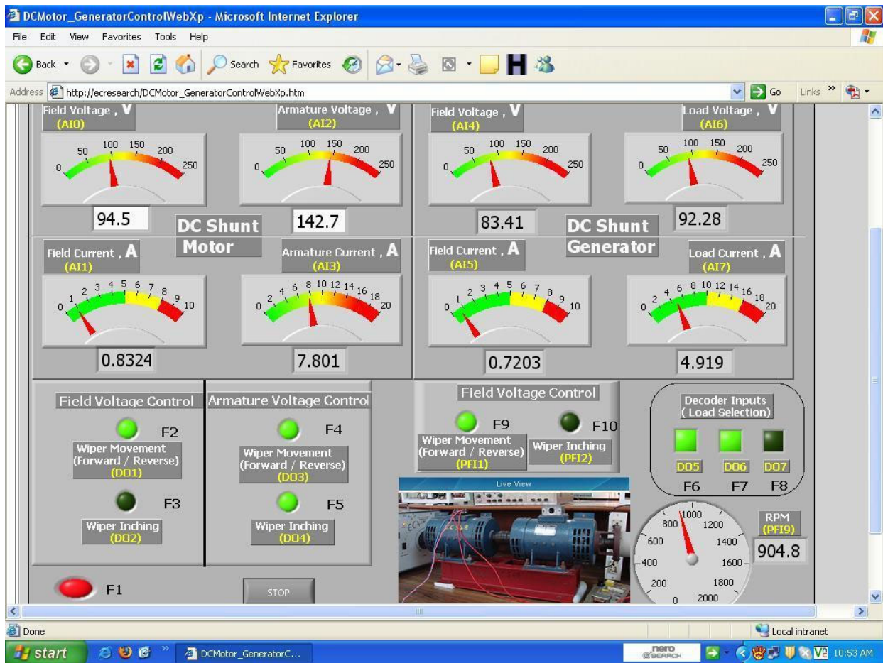
Figure 4. Web page of the front panel along with live view of experiment hardware
