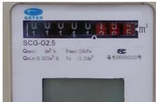
**Fig. 7.** Meter with failed reading
