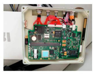
Fig. 3. Hardware circuit of smart operation and maintenance box
