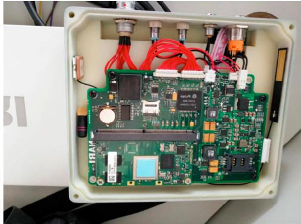
**Fig. 3.** Hardware circuit of smart operation and maintenance box
