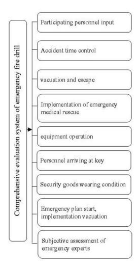
Fig. 9. Comprehensive evaluation module for emergency fire drill
