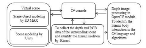
Fig. 1. The system data flow
