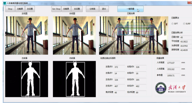
Fig. 9. The interface of body height estimation system
