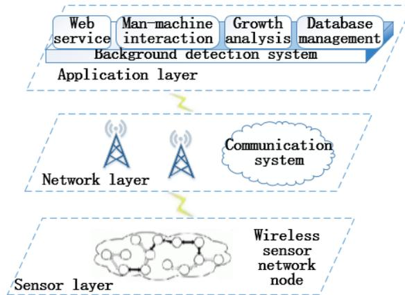
Fig. 6. Sugarcane growth monitoring analysis system framework
