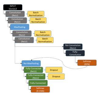
Fig. 3. Faster R-CNN Architecture
