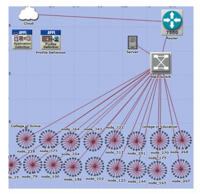
Fig. 1. The university campus main design without firewall
