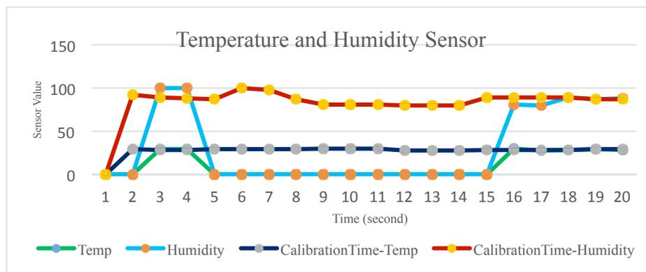
**Fig. 6.** The result of calibration time for temperature and humidity sensing element.
