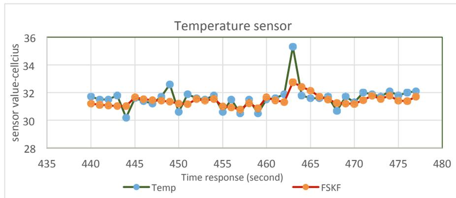
Fig. 8. The FSKF with a temperature detector.
