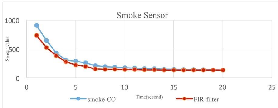
Fig. 7. Self-calibrate by FIR filter.
