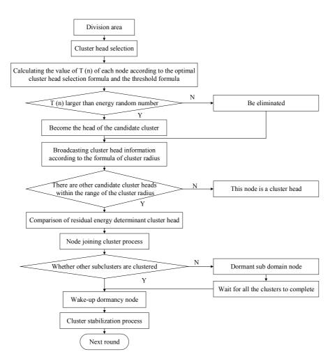
Fig. 7. Formation process of cluster data fusion based on residual energy dormancy scheduling
