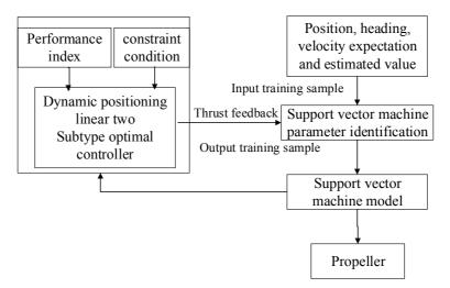
Fig. 3. The schematic diagram of the support vector MPC controller
