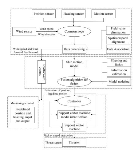
Fig. 1. General flow chart of ship dynamic positioning control system
