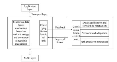
Fig. 6. The data fusion mechanism independent of the application
