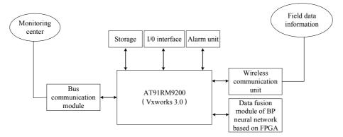
Fig. 2. The structure of the convergence node of the ship dynamic positioning system
