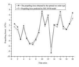
Fig. 5. The prediction error of the longitudinal control force of the ship
