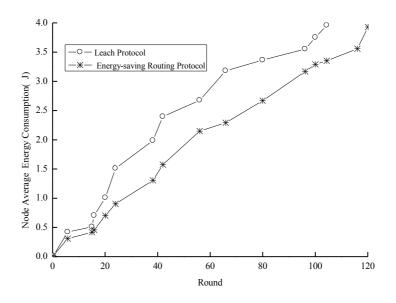
Fig. 9. The comparison of the average energy consumption
