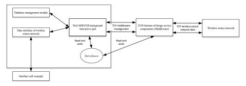
Fig. 2. The relationship between wireless sensor network and Web service
