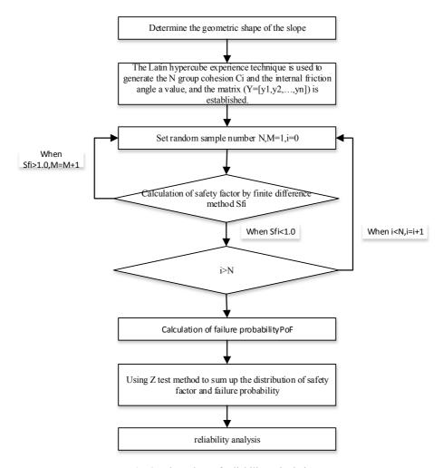
Fig. 3. Flow chart of reliability calculation
