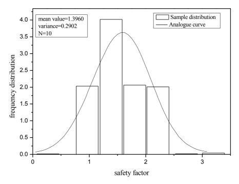
**Fig. 4.** N=10 safety coefficient frequency histogram
