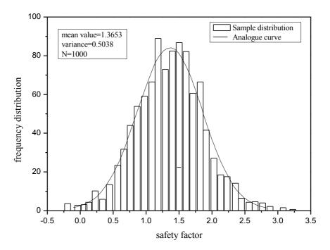
Fig. 6. N=1000 safety coefficient frequency histogram
