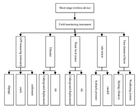
Fig. 1. Structure of multi parameter monitoring instrument
