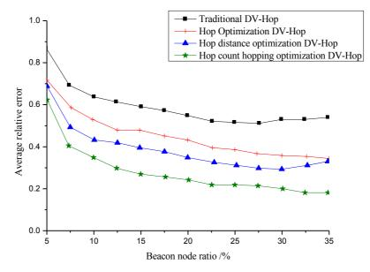
Fig. 7. Comparison of relative positioning errors of three improved algorithms
