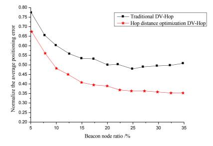
Fig. 6. SquareDeviationRelativePositioningErroroftheRatioofDifferentBeacon
