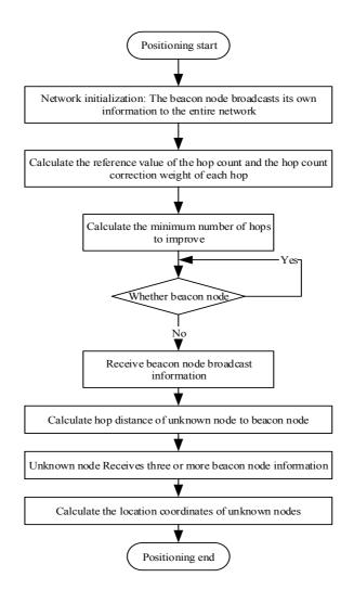
Fig. 2. Improved DV-Hop Location flow chart based on minimum hops
