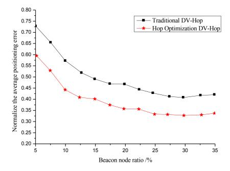
Fig. 5. Square Deviation Relative Positioning Error of the Ratio of Different Beacon
