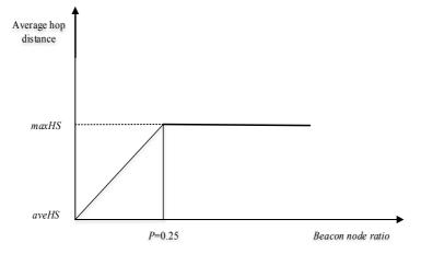
Fig. 4. Relationship between Beacon Node Ratio and Average Hop Distance
