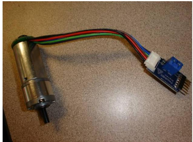
Figure 12. PmodHB5 module with motor attached
