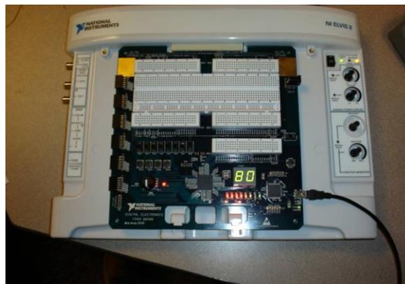
Figure 1. NI-ELVIS II platform with the Digital Electronics FPGA Board
