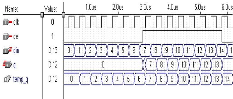
Fig. 8. Simulation waveform of Lock
