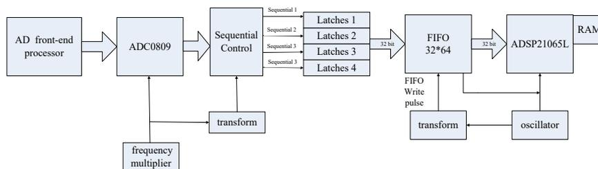
Fig. 1. Block diagram of data acquisition
