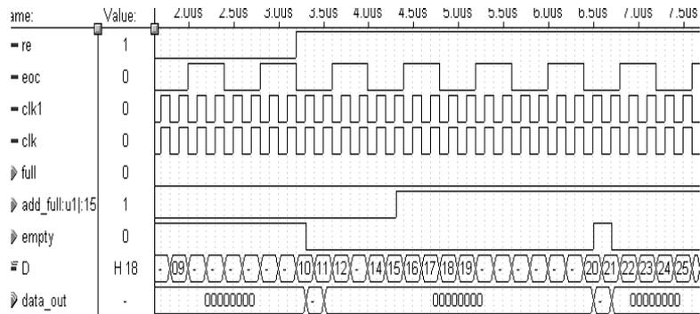
Fig. 3. The simulation waveform of this overall system program
