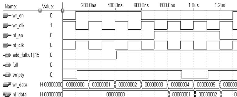
Fig. 12. Simulation waveform of FIFO
