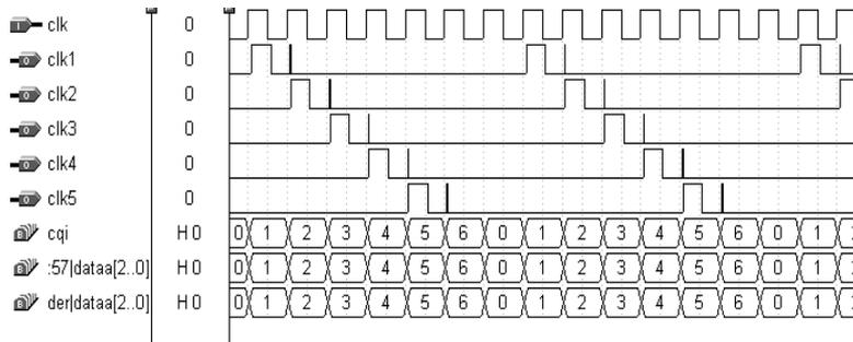
Fig. 10.Simulation waveform of clock conversion module
