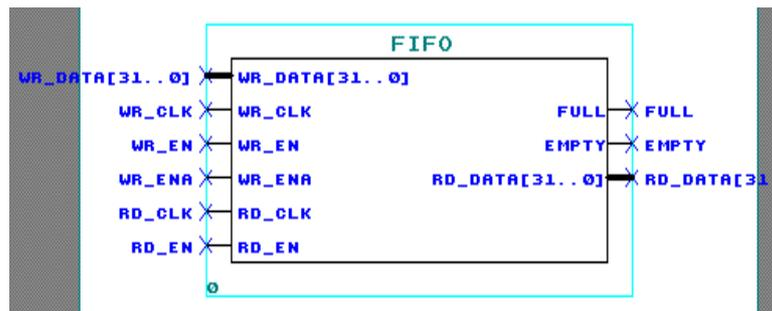
Fig. 11. FIFO module circuit design
