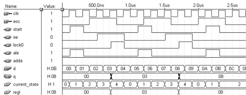
Fig. 4. Simulation waveform Control Module Design for ADC0809 Chip
