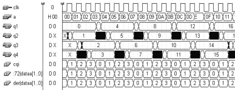
Fig. 6. Simulation waveform of data allocation module
