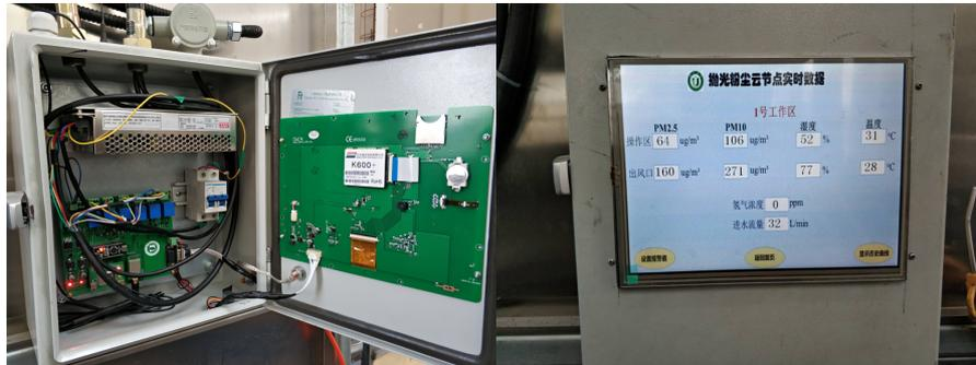
Fig. 13.Sink node with HMI
