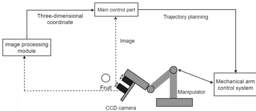
Fig. 2. The schematic diagram of the fruit recognition system for the target of the picking robot
