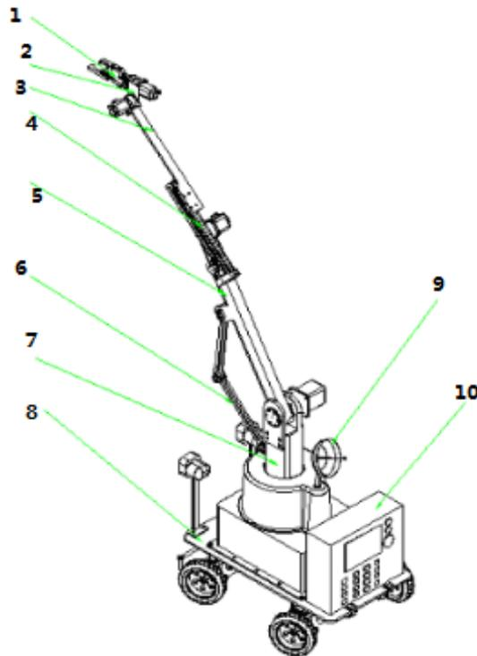
1. The end-effector 2. The CCD camera 3. The small arm component 4. The servo motor 5. The large arm component 6. The larger arm auxiliary component 7.the main arm 8. The vehicle acoustic carrier 9. The sensor module 10. The main control part
