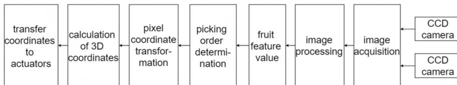
Fig. 6. The work frame diagram of visual system for picking robot
