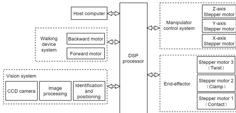
Fig. 3. The circuit control frame diagram of target fruit recognition system
