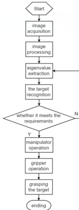
Fig. 4. The schematic diagram of the software flow of the intelligent picking robot system
