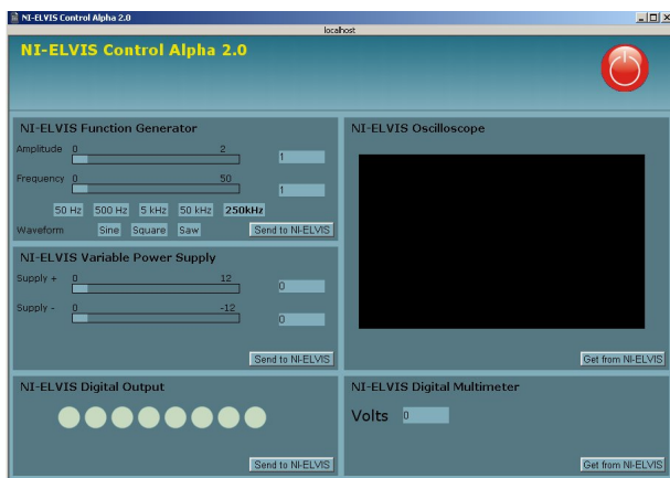
Figure 3. The goal of this version was to include linear potentiometers in an effort to make the interfaces as similar to an actual device as possible
