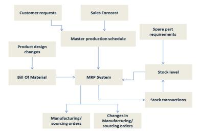
Fig. 2. MRP process flow diagram
