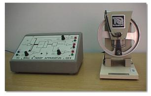
Figure 3. Photograph of the Ball & Hoop System
