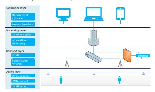
Fig. 4. Structure of the UWB-WSN monitoring platform
