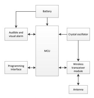
Fig. 5. Hardware structure of location tag
