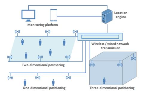
Fig. 2. Structure of UWB-WSN
