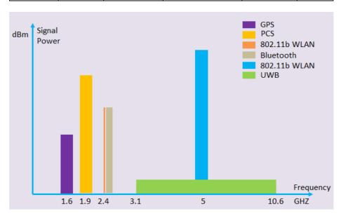
Fig. 1. Spectrum and power of different short-range wireless positioning technologies
