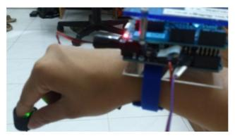
Fig. 21.ECG signal monitoring device, sender module.
