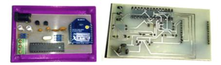
Fig. 11. Zigbee module and microcontroller unit, front and back.
