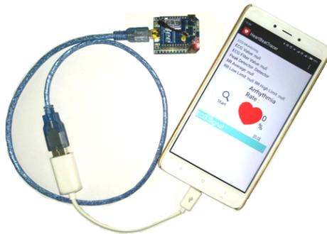
Fig. 16. The connection of Zigbee module and Smartphone by USB OTG cable.
