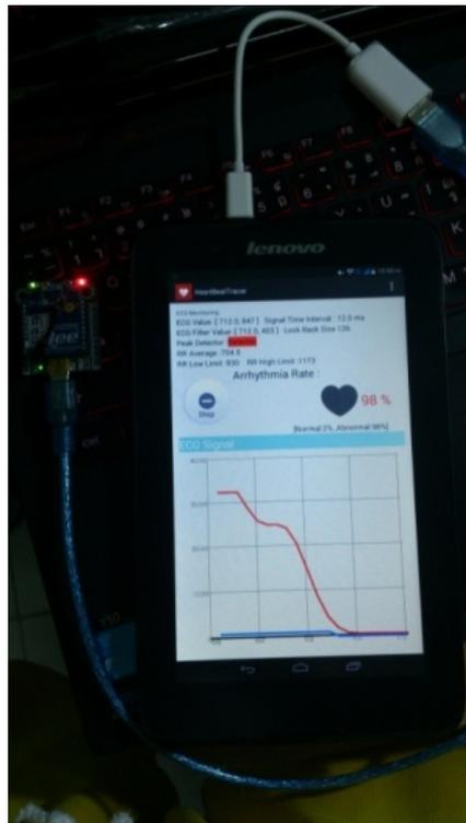
**Fig. 22.** The ECG signal data receiver connected to Smartphone.
