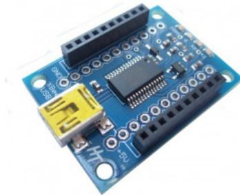
Fig. 13. Mini Xbee USB Dongle for Zigbee module programming.
