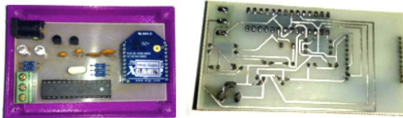
Fig. 11. Zigbee module and microcontroller unit, front and back.
