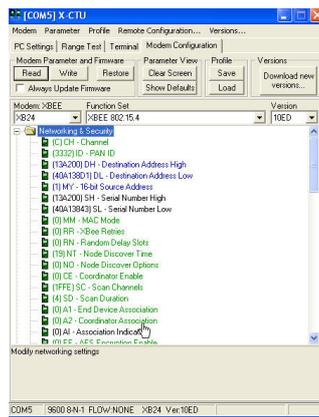
Fig. 14. Zigbee management by X-CTU
