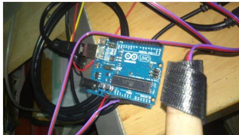
Fig. 15. Figure 3-11 Detect the ECG signal by ECG sensor.
