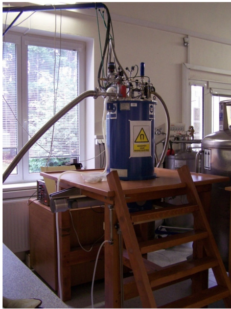
Figure 7. Mössbauer spectrometer for low-temperature and in-field measurements (Spectromag system, Oxford Instruments)
