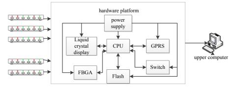
Fig. 1. Overall block diagram of grating slope detection system
