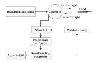
Fig. 4. Tunable fiber F-P filter method
