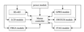
Fig. 6. Hardware circuit module diagram
