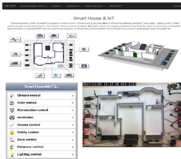
Fig. 8. Remote Lab Smart House & IoT web-interface
