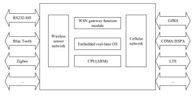
Fig. 3. The architecture of WSN gateway platform
