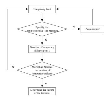
Fig. 6. Terminal fault management flowchart
