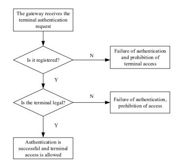
Fig. 5. Authentication processing flow chart
