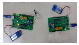
Fig. 7. Physical map of point-to-point communication sensor data acquisition system
