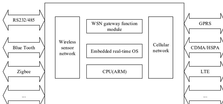
Fig. 3. The architecture of WSN gateway platform
