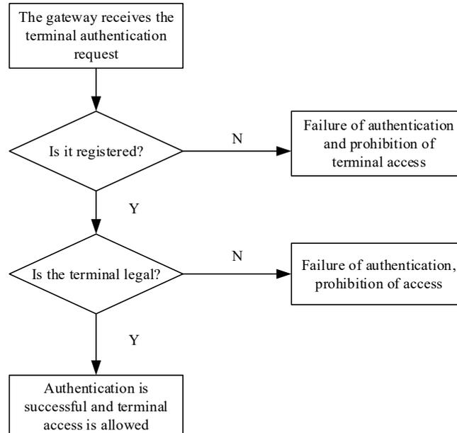
Fig. 5. Authentication processing flow chart
