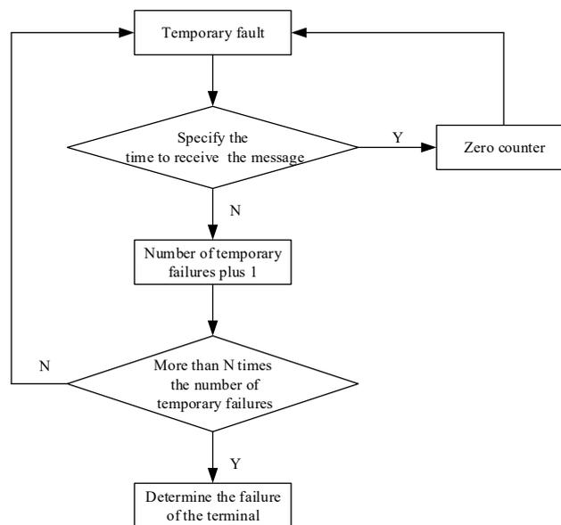
Fig. 6. Terminal fault management flowchart
