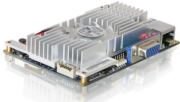
Figure 4. The software add-on: x86-compatible VIA board for all computational-intensive applications [6]
