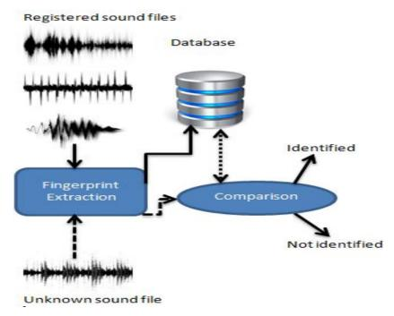
Fig. 1. General architecture of an acoustic identification system based on fingerprinting
