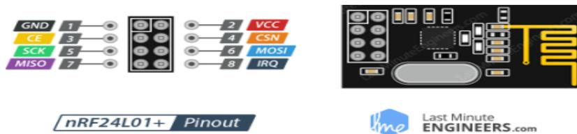
**Fig. 6.** Pinout of nRF24L01
