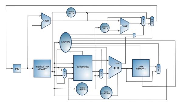
Figure 2. Functional units of the datapath defined for the MIPS X-Ray plug-in.
