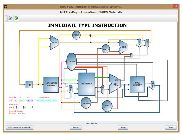
Figure 5. Execution of the immediate type instruction in the Mips X-Ray plug-in.
