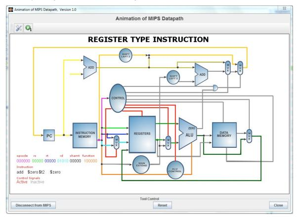
Figure 3. Execution of the register type instruction in the Mips X-ray plug-in.
