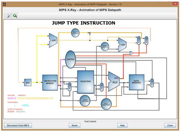
Figure 4. Execution of the jump type instruction in the Mips X-Ray plug-in.
