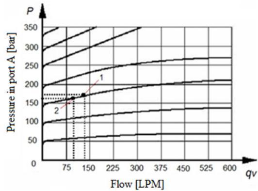
Figure 2. Typical curve of steady state of a relief valve [4]
