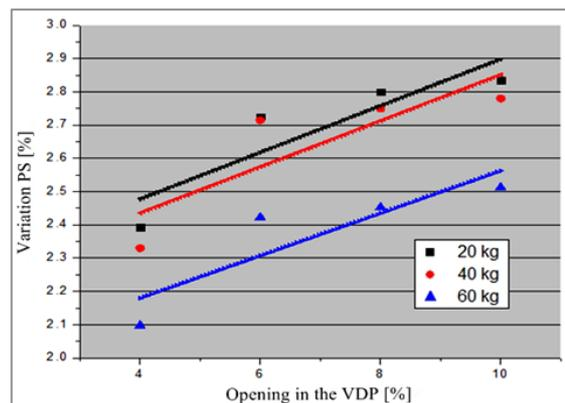
Figure 11. Variation of  $P_S$  x aperture VDP (using the accumulator in the circuit).
