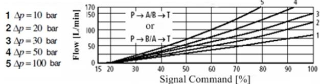
Figure 5. Graph command signal versus of a flow proportional valve [4].
