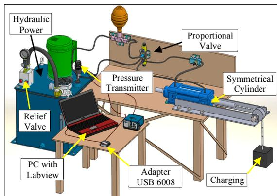
Figure 3. Components of the bench study
