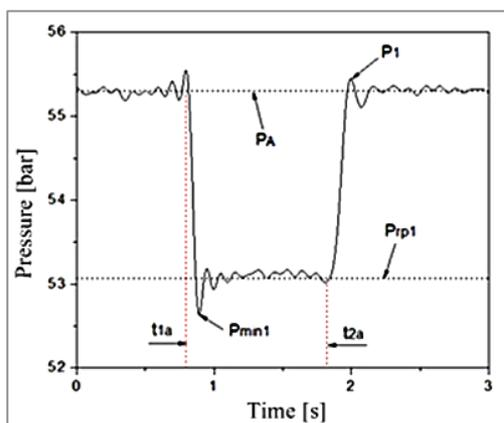
Figure 6. Dynamic behavior of supply pressure without the use of the accumulator with opening of 100% in the VDP.
