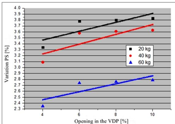
Figure 10. Variation of  $P_S$  x aperture VDP (not using the accumulator in the circuit).
