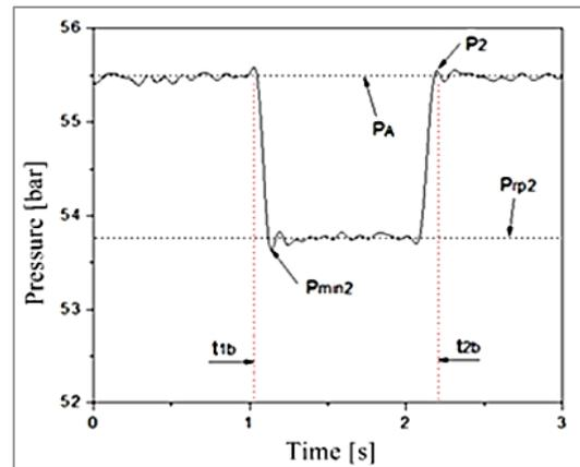
Figure 7. Dynamic behavior of supply pressure without the use of the accumulator with opening of 40% in the VDP.
