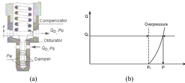
Figure 1. Principle of operation of the pressure relief valve, direct operated. (a) the constructive-way [1] e (b) static feature [10]
