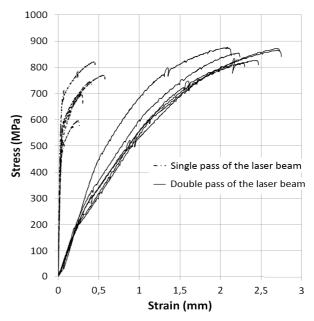
Figure 2. Tensile curves for both of the sample groups
