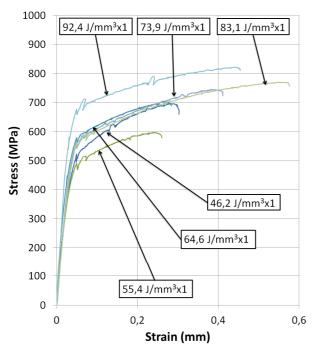
Figure 3. Tensile curve diagrams obtained for the samples on which one laser beam pass over each patch was used.
