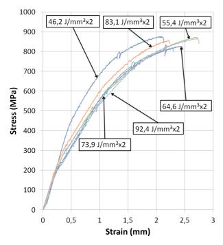
Figure 4. Tensile curve diagrams for the samples on which two laser beam passes over each path were used.
