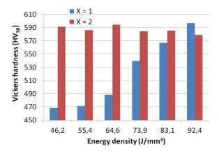
Figure 6. The mean values of the Vickers hardness  $(HV_{30})$  obtained for all of the sample variants.
