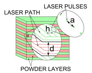
Figure 1. The SLM process scheme: a – distance between the laser beam pulses, h – distance between the laser beam paths, d – thickness of single layer
