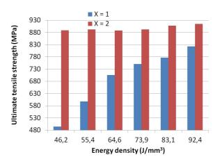
Figure 5. The mean values of the ultimate strength (Rm) obtained for all of the sample variants.
