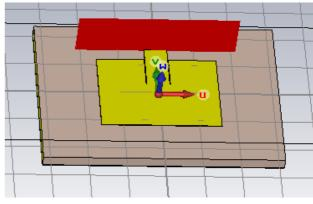
Figure 2. Designed Microstrip Patch Antenna for 5.8 GHz.
