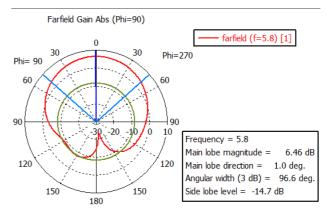
Theta / Degree vs. dB Figure 8. Far field in polar view for RTDuroid 5880.
