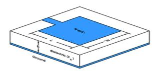
Figure 1. Structure of Patch antenna [3].
