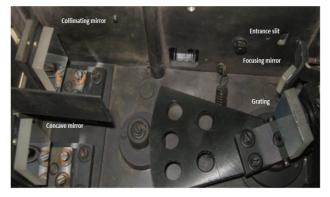
Figure 2. Picture of the optical system based on the Czenry turner configuration
