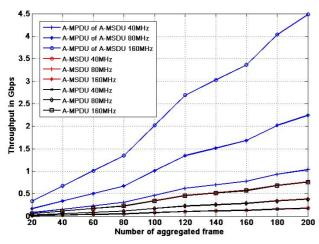
Figure 7. Throughput for the RTS/CTS access scheme
