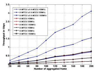
Figure 6. Throughput for the basic access scheme
