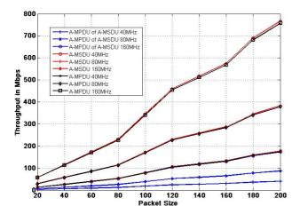
Figure 8. Throughput against the packet size
