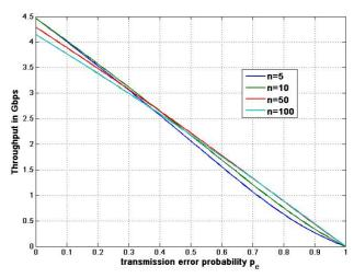
Figure 5. Throughput vs. Transmission error probability
