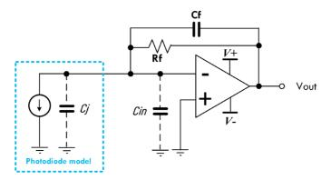
Fig. 1. TIA model, the figure is reproduced version from the original article at [26], [53]
