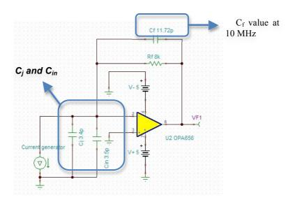
Fig. 2. TIA circuit in TINA<sup>TM</sup>-SPICE® in OPA656 simulation case
