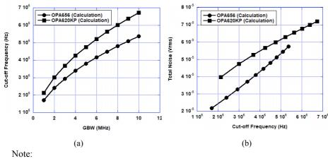
$f_{-3dB}$  is calculated using Eq. 2  $N_{tot}$  is calculated using Eq. 1
