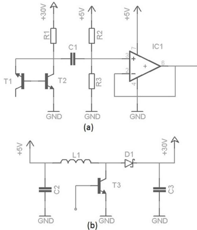
**Fig. 8.** Noise generator circuit (a) and boost converter (b)
