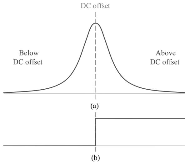
**Fig. 5.** Comparator output (b) depending on the noise signal input (a)
